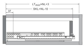
LT<sub>min</sub>:Inside Cabinet Depth(Min.)
